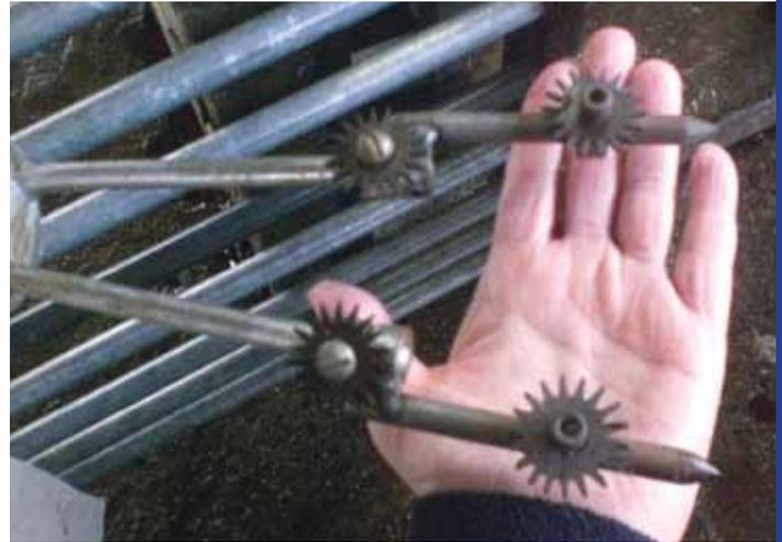
For animals over 200 lbs: use Wand Extension tips and Stainless Steel Spurs to assure correct Stun Wand contact. Note: Stainless Steel Star Wheels (spurs) conduct better than carbon steel.
